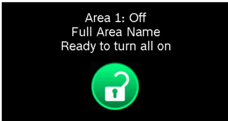
The Main icon serves as both an indicator of the arming state and alarms, and as an icon to press to change the arming state. The text above the icon provides instructions.
